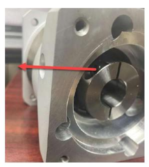
motor shaft is aligned with the access hole. Loosen the set screw and remove the 4 screws that hold the motor on. On the bottom of the gantry remove the 4 3/8" bolts holding the cover on. Slide the motor into the gear box and fasten the motor using the 4 supplied screws you took out of the gear box. Next, remove the plug for
